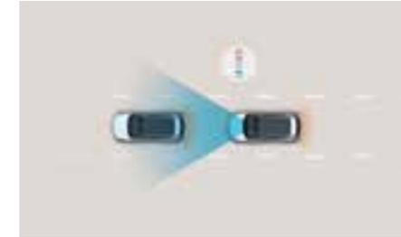
**Forward Collision-Avoidance Assist (FCA) with pedestrian detection.** The FCA system uses the front mounted camera and the radar sensor to monitor the traffic ahead. Should it detect a potential collision with a vehicle in front or with a pedestrian, it will warn the driver and if required, automatically slow or stop the vehicle.
