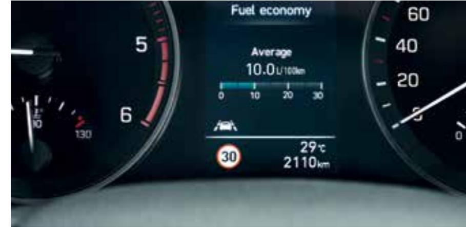
**Supervision cluster** – Optimally placed and easy to read, the supervision cluster with its 4.2" colour LCD screen shows important driver information like: the status of active safety features, remaining range, fuel consumption, navigation instructions, outside temperature and more.
