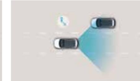
**Blind Spot Collision Warning (BSCW) with Lane Change Assist (LCA).** Using 2 radar sensors in the lower rear bumper, the system visually warns you of traffic in the blind spot area. Should you set the turn indicator in such a situation, the Lane Change Assist will sound an acoustic alert.
