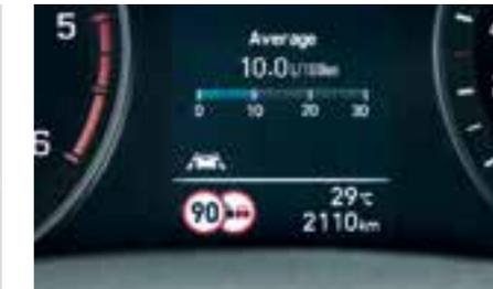
**Intelligent Speed Limit Warning (ISLW).** The Intelligent Speed Limit Warning uses the front camera and information from the navigation system to identify road speed signs and displays the speed limit and no-passing signs in real time. The information is displayed in both the navigation system display and the TFT cluster.
