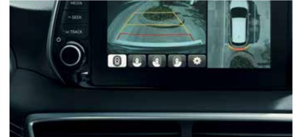
**Surround View Monitor** – Nice and easy. The Surround View Monitor in the New Tucson helps make manoeuvring in confined spaces easier and safer. Through a series of strategically located cameras, this advanced safety feature provides you a 360° view of the area surrounding the vehicle so you can see exactly what you're doing.
