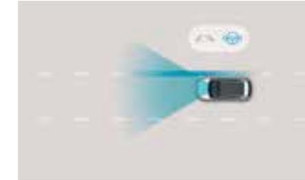
**Lane Keeping Assist (LKA).** The standard LKA uses the front camera to monitor the lines of the road. In case of an unintended lane departure, it will warn the driver and can apply counter steering torque to guide the car back to the lane.
