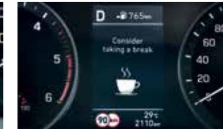
**Driver Attention Warning (DAW).** This standard feature raises safety and convenience to an entirely new level by continuously monitoring and analysing driving patterns. When a pattern of fatigue or distraction is identified, DAW gets the driver's attention with an audible alert and pop-up message suggesting a break.
