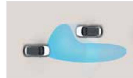
**Full LED Lighting Technology.** High Beam Assist detects oncoming vehicles as well as vehicles in the same lane ahead at night, and changes from high beam to low beam as appropriate. The Static Bending Light illuminates the front side area ahead when cornering, improving visibility at night.
