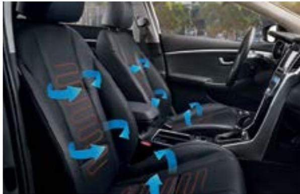
**Heated & ventilated front seats.** When it's cold outside, nothing is more welcoming than a heated seat. And you'll appreciate the cooling effect of seat ventilation on summer journeys. Both have 3-stage adjustment.
