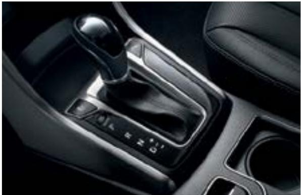
**Dual-Clutch Technology.** The 7-speed Dual-Clutch Transmission (DCT) brings distinct benefits to both performance and fuel efficiency. Standard with both versions of the 1.6 diesel engine and the 1.6 GDI petrol engine.
