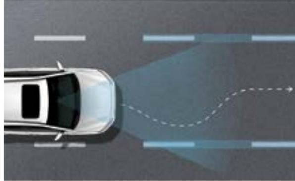
**Lane Keeping Assist (LKA)** The standard LKA uses the front camera to monitor the lines of the road. In case of an unintended lane departure, it will warn the driver and can apply counter steering torque to guide the car back to the lane.
