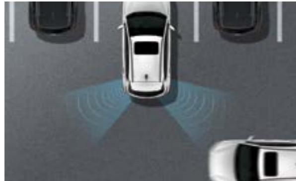
**Rear-Cross Traffic Collision Warning (RCCW)** When reversing out of a narrow parking space, the Rear-Cross Traffic Collision Warning reduces the risk of a collision. Using 2 radar sensors at the rear, it warns you in case of any approaching cross traffic.
