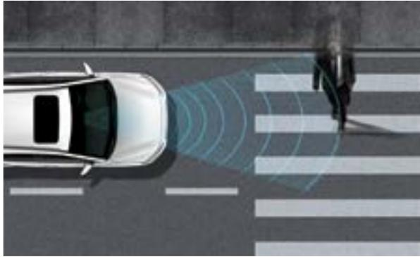
**Forward Collision-Avoidance Assist (FCA) with pedestrian detection** The FCA system uses the front mounted camera and the radar sensor to monitor the traffic ahead. Should it detect a potential collision with a vehicle in front or with a pedestrian, it will warn the driver and if required, automatically slow or stop the vehicle.
