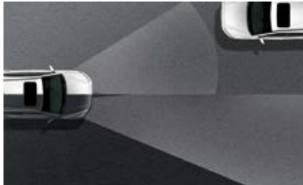
**Full LED Lighting Technology** High Beam Assist detects oncoming vehicles as well as vehicles in the same lane ahead at night, and changes from high beam to low beam as appropriate. The Static Bending Light illuminates the front side area ahead when cornering, improving visibility at night.
