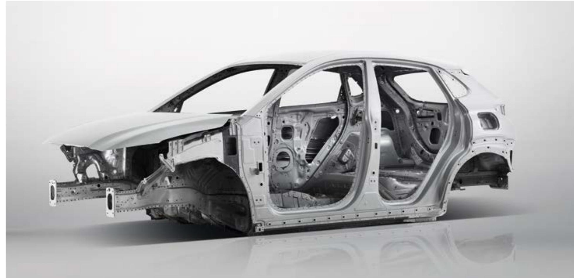
The all-new KONA benefits from superior rigidity through the use of advanced high strength steel and high impact energy absorption that protects passengers in the event of a collision. The structure of the cabin is designed to disperse energy in the event of a collision, therefore reducing impact to occupants.
