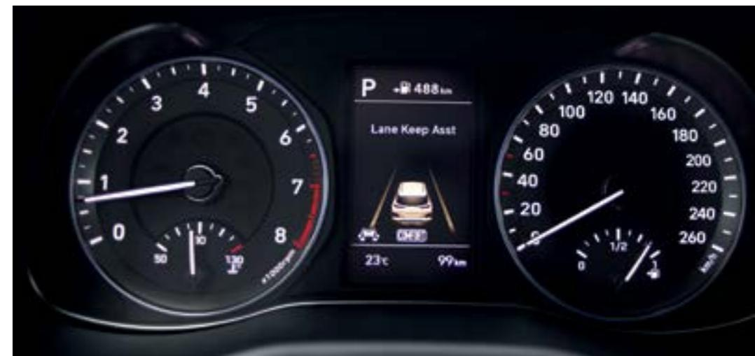
Digital Information Cluster – Optimally placed and easy to read, a 4.2" LCD screen shows you important driver information like: the status of active safety features, remaining range and fuel consumption, navigation instructions, outside temperature and more.
