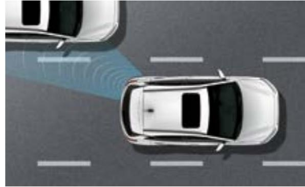
**Blind Spot Collision Warning with Lane Change Assist** Using 2 radar sensors in the lower rear bumper, the system visually warns you of traffic in the blind spot area. Should you set the turn indicator in such a situation, the Lane Change Assist will sound an acoustic alert.
